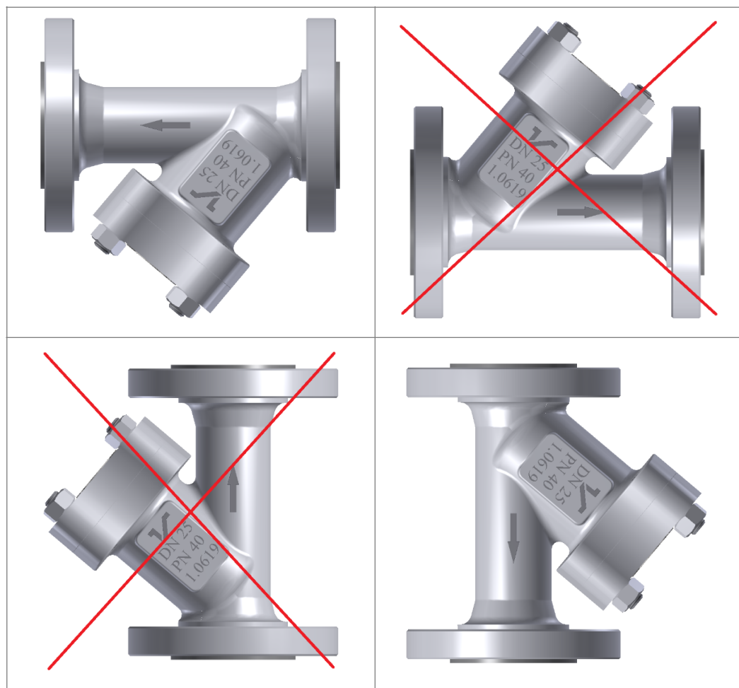
Fig. 2 Recommended mounting position
