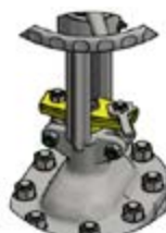
Figure D.2.26 – Stem packing gland tightening
